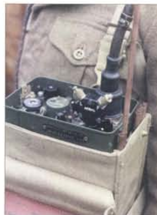
Fig. 4: The antenna unit for longer whips and wires. Note the rubber boot over the rear connector.
