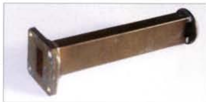
Fig. 4: The G4ALN Penny Feed, the slots cut in the 'long' side are 14.5x1.5, and the 'cap' has a diameter of 30mm (almost the same size as an old English penny).
