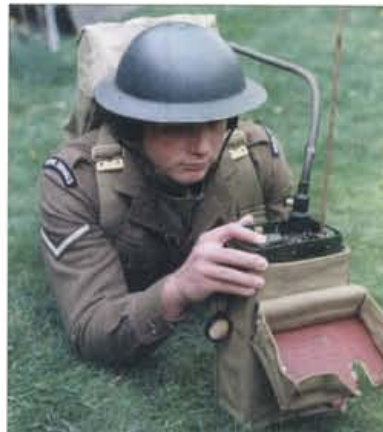
Fig. 3: The operating position on the ground. The set unclips from the belt and is placed flat on the ground.
