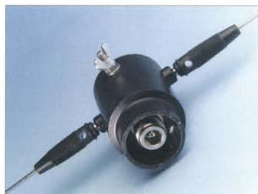
Fig. 3: An N-type plug set into a plastic block forms the centre of a portable dual-band dipole.
