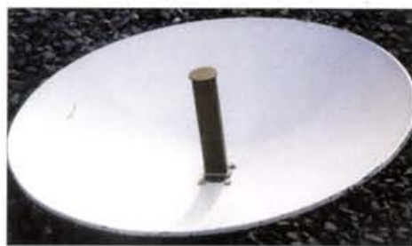
Fig. 5: A 460mm diameter dish (originally made for the PW EXE) with penny feed.
