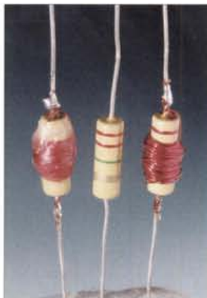
Fig. 3: Winding 'home-brewed' radio frequency chokes on resistor bodies (see text).
