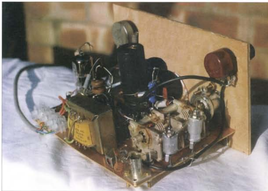
Fig. 3: Rear 'chassis' view of the G4HUV project. The prototype uses a plywood front panel with a p.c.b. material main 'chassis'.
