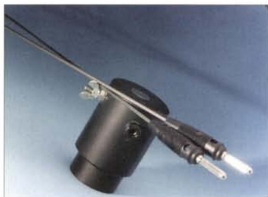
Fig. 4: Two 4mm plug/socket arrangements are used for mounting the elements of the antenna.
